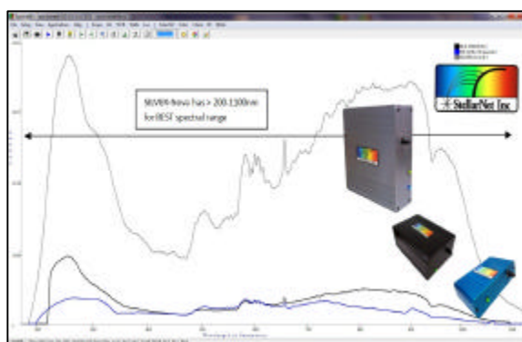
Reference Spectra of Deuterium + Halogen lamps using SL5-DH source
