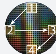
Automated sampling at each location results in multiple measurements from one loading of the stage
